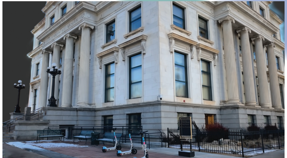
Figure 1. 3DGS reconstruction of the Legislative Services Building (historically known as the Colorado State Museum, built 1915) from gimbaled smartphone video. Note the fine architectural detail captured in the ornamental railings and the photorealistic rendering of reflective glass windows, demonstrating 3DGS capabilities for heritage documentation.
